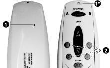
2. While the Indicator Light is flashing green, press the group button for the group to which you plan to assign the shade.
