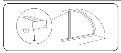
(1) Mount the top clip at the top center of the arch opening.
