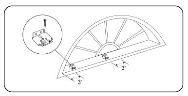
**Shades stacking on the left**, mount one installation bracket approximately 3" from the left side of the opening and the other bracket 3" to the left of the center of the window opening.
