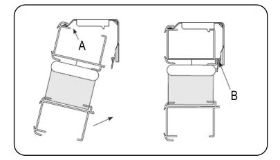
Start with the top rail (the rail with the motor in it). Make sure that the receiver wire is out of the headrail before mounting. Position the receiver wire so that it is facing into the room and position the motor wire so that it comes out the back side of the shade, ensuring it is not pinched by the bracket.
