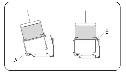
Position the rail with the front lip (A) resting on the hooks of all the brackets. Push the rail firmly down and toward the window until the groove on the rail snaps into place, (B) as shown.
