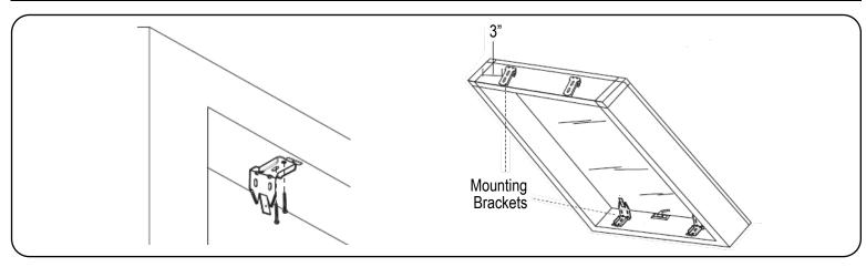
Using the mounting bracket (included) as a template, measure to the edge of the bracket and mark the hole locations with a pencil for drilling. End brackets should be located approximately 3" from either end. Use a 3/32" drill bit to drill holes for the screws. Depending on the width of the shade, additional brackets may be necessary, evenly spaced between the two end brackets.
