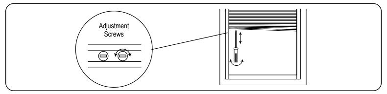
If the moving rail is uneven it can be leveled using the shade adjust on the bottom of the rail. Use a flat head screwdriver or a dime to turn the adjustment screw to raise or lower that side of the bottom rail. The adjustment screw is on the bottom of the moving rail. One quarter turn of the screw will move the moving rail up or down approximately 1/4"
