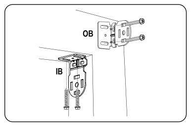
Secure the roller shade installation brackets with the supplied screws. If shade was ordered as outside mount (OB), attach the supplied screw covers on to the bracket for a finished look.
