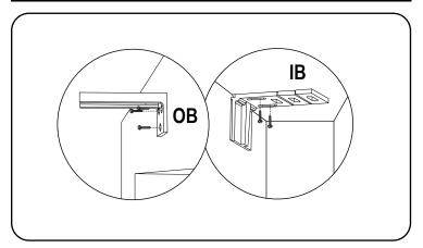
Outside mount (OB) requires a T-Bracket installation. Space brackets evenly. **Note:** *Do not attach the Deco Fascia until the shade has been installed.*
