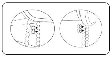
**Upper Limit**, pull the back chain until the desired upper position. Then, snap the chain stop to the bead just below the clutch.
