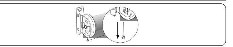
Important: Do not to pull the lock pin until shade is securely assembled onto the brackets.
