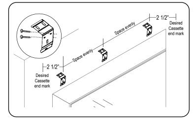
Inside Mount, install the brackets level and aligned to each other, using the screws provided.
